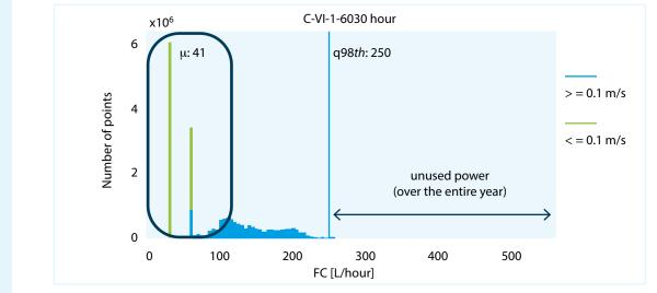
These quantitative insights on the impact of downstream vessel speed and installed engine power provide inland shipping operators with perspectives for action to reduce ship emissions on their own in the future.
