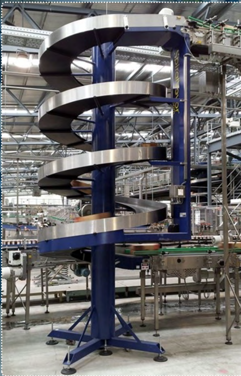
Spiral conveyors over 30 metres, Apollo
